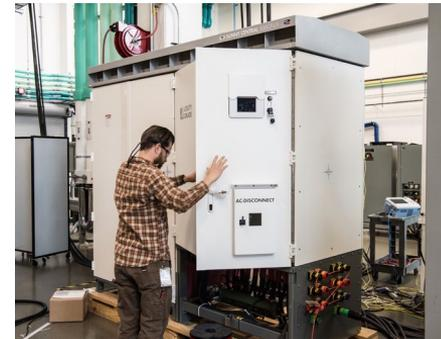
HIL test setup with real-time digital simulators, PV inverters, and advanced microgrid controllers
