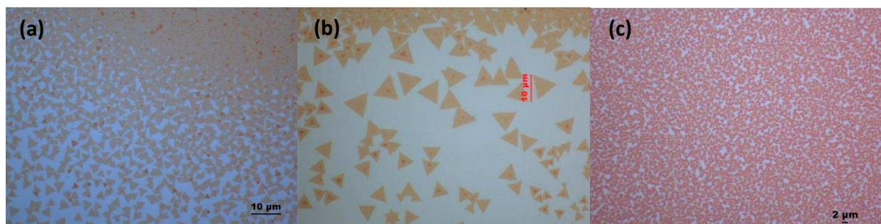
Figure 4. Optical images comparing maximum reaction temperature hold time. (a) 5 minutes. (b) 3 minutes. (c) 2 minutes.
