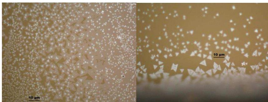
Figure A2. MoS<sub>2</sub> flakes on quartz substrate. Conditions of 700°C for 3 minutes, 760 torr pressure, and 200 sccm gas flow rate were successfully used to grow single and few layer crystals on substrates other than Si/SiO<sub>x</sub>.
