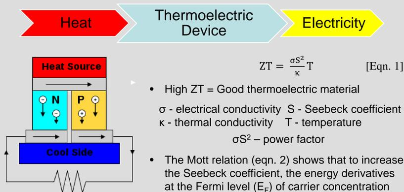
Schematic of a thermoelectric device. (wikipedia)
