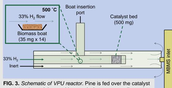
**FIG. 3.** Schematic of VPU reactor. Pine is fed over the catalyst at a 1:1 ratio, and the resulting pyrolysis vapors are directed to a molecular beam mass spectrometer (MBMS) for analysis.
