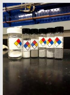
**Catalyst synthesis:** Metals were added to ZSM-5 via incipient wetness impregnation at a constant molar ratio of 1:2 metal-to-aluminum.
