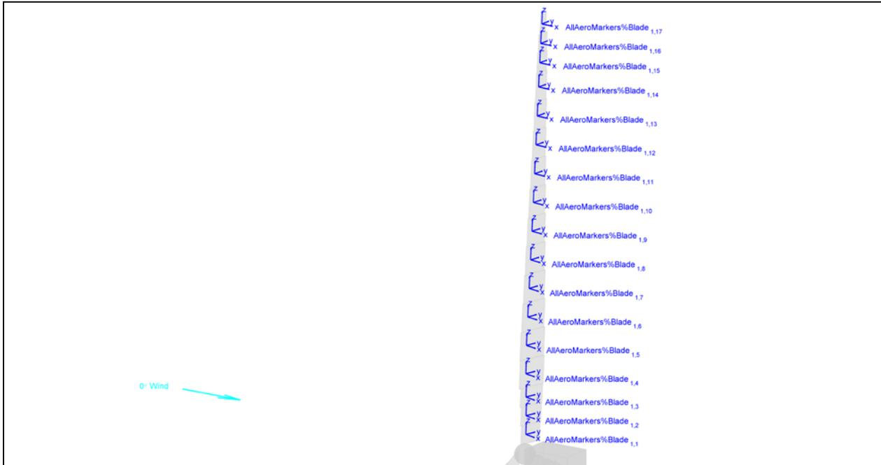
**Figure 10. Schematic of AllAeroMarkers%Blade markers for Blade 1 of the NREL 5-MW Baseline Onshore Turbine. This blade has 17 aerodynamic analysis nodes.**
