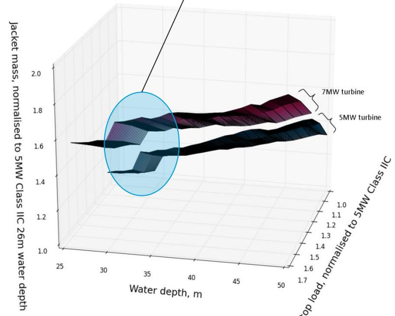
Jacket mass  $\sim 20\%$  increase from class C to class A.  $\sim 20-30\%$  increase from 26m to 50m water depth
