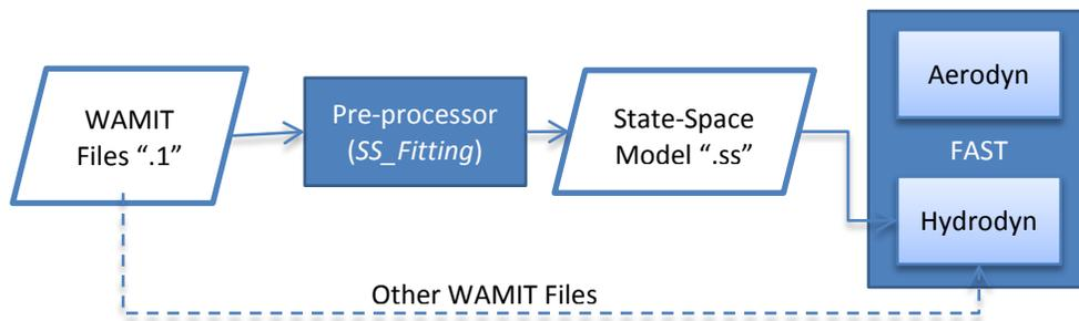
FIGURE 5: MATLAB PRE-PROCESSOR AND REQUIRED FILES.
