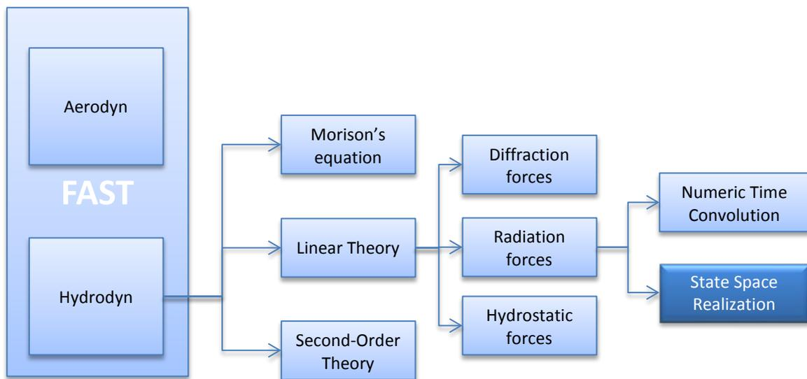
FIGURE 1: HYDRODYN MODULES INCLUDING THE NEW STATE-SPACE REALIZATION MODULE.
