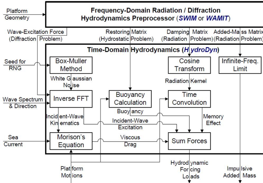
FIGURE 2: SUMMARY OF THE CALCULATIONS FOR THE INTERFACE OF SUPPORT PLATFORM LOADS TO FAST AND ADAMS. (JONKMAN & BUHL, 2007)
