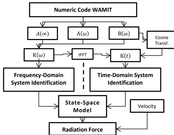
FIGURE 3: SCHEME OF THE RADIATION FORCE CALCULATION USING FREQUENCY- OR TIME-DOMAIN IDENTIFICATION METHODS.
